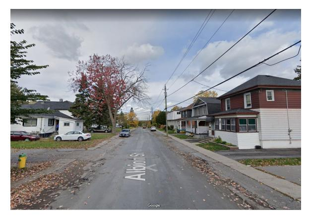
Storm water is managed via overland flow through paved shoulders, channeling water to the north  Asphalt and paved shoulders are in poor to very poor condition
